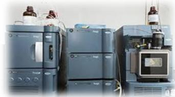
Exion LCTM AC System (AB Sciex) and a Triple Quad<sup>TM</sup> 3500 system (AB Sciex) in ESI negative ionization
